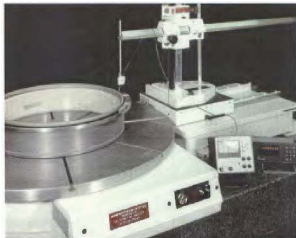
100mm diameter air bearing rotary table used for measuring applications
