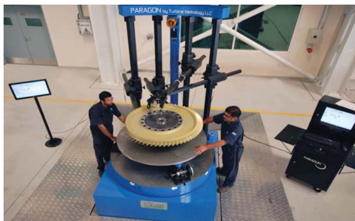
Circular geometric inspection system
