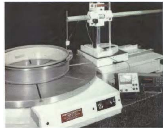
100mm diameter air bearing rotary table used for measuring applications
