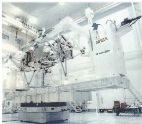
4,000mm diameter air bearing rotary table used for satellite assembly
