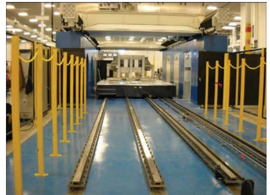
4 meter x 7 meter twin pallet system used in aerospace manufacturing.
